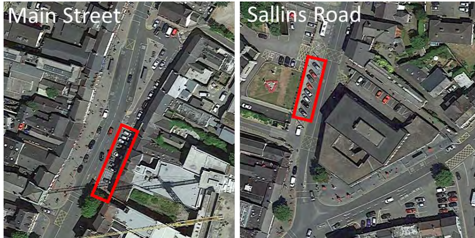
Figure 9.24 Parking Option 2: Relocate Perpendicular Parking
