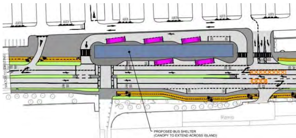
Figure 8.2 Example of a Bus Interchange: Draft Design of Proposed Blanchardstown Transfer Hub
